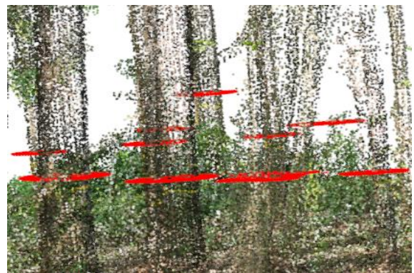
Fig1 DBH detection in thinned point cloud
